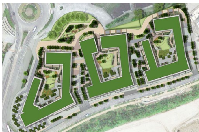
First Central, Lakeside Drive Scheme amended to deliver 75% of roof level surface as extensive (0.7) green roof. UGF = 0.41
