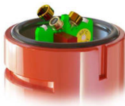
Figure 12 Optical filters in a detector
